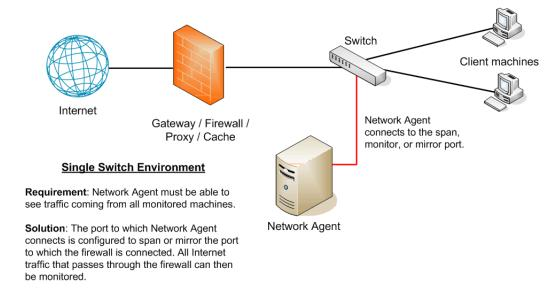
If you use a switch that supports bidirectional spanning (allowing packets to be monitored and sent from the same port), Network Agent needs only one NIC.
