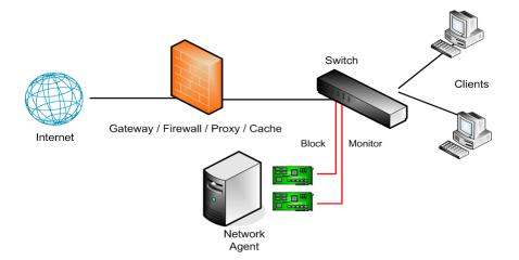
Each NIC that Network Agent uses for monitoring must be able to see all inbound and outbound traffic for the network or segment that it is configured to monitor.
