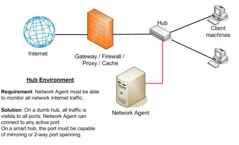
Network Agent must see the traffic, in both directions, for those segments of the network that it is assigned to monitor. The port to which the Network Agent machine is attached must be capable of bidirectional port spanning (mirroring).
